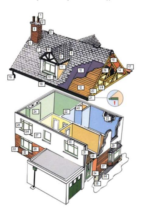
3 Chimney head 4 Flashing Ridge ventilation 5 6 Ridge board Slates/tiles 8 Valley guttering 9 Dormer projection 10 Dormer flashing 11 Dormer cheeks 12 Sarking 13 Roof felt 14 Trusses 15 Collar 16 Insulation 17 Parapet gutter 18 Eaves guttering 19 Rainwater downpipe 20 Verge boards / skews 21 Soffit boards 22 Partition wall 23 Lath / plaster 24 Chimney breast 25 Window pointing 26 Window sills 27 Rendering
